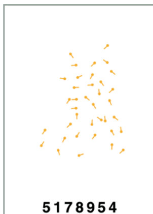
The minutiae are transformed into a group of figures by means of an algorithm. This means that no images of the fingerprints are stored but pure groups of figures.
